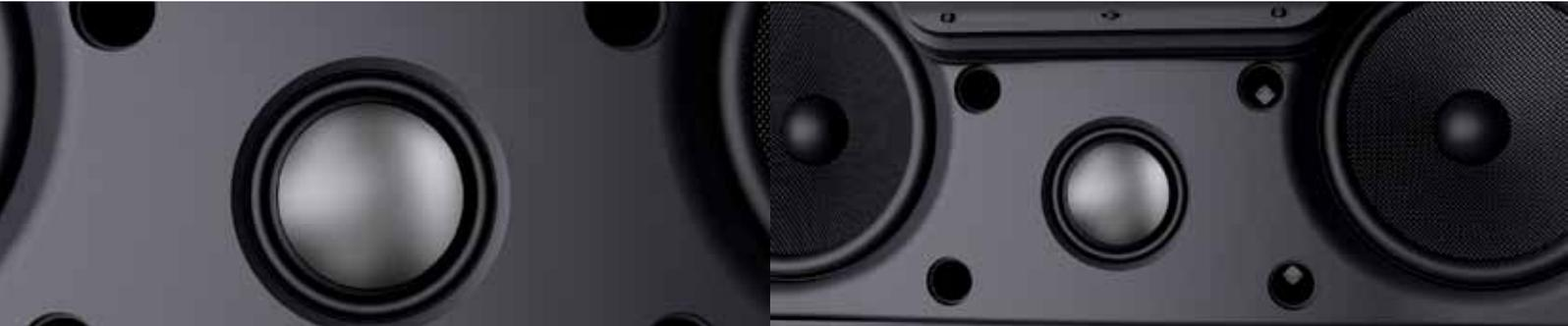
**Tweeters** Panorama 2 uses aluminium dome Nautilus™ tube-loaded tweeters. The elongated shape swallows unwanted noise behind the dome. The same technology is found in our audiophile hi-fi speakers, such as the reference-standard 800 Series Diamond. And the tweeters have now been improved in Panorama 2 for better crossover with midrange drivers.
